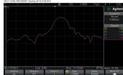
Spectrum signal comparison. (CF 900 MHz; span1 MHz; RBW 1 kHz (MDO3104), 19.1 kHz(X3104A)). MDO3000 also offers automatic markers and spectrogram display.
