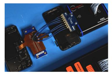
Typical Application: Form Factor Probing of MIPI-Based Designs
