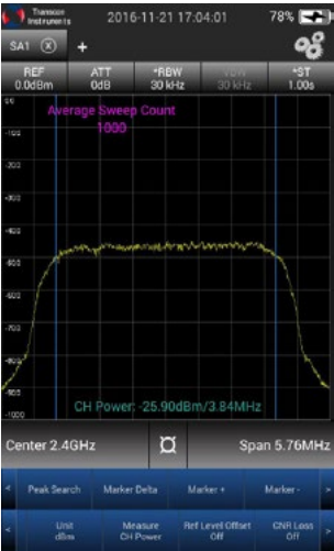
Channel power measurement
