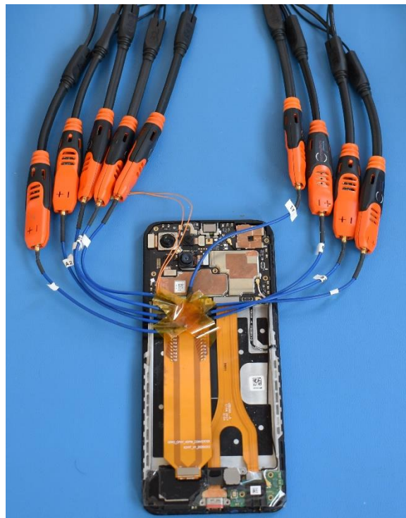
Figure 3: Typical PV1 application: monitoring live traffic on a phone
