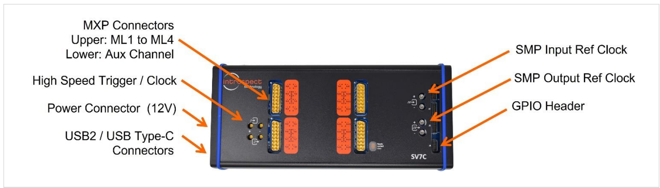
Figure 2: SV7C-eDP physical connections.
