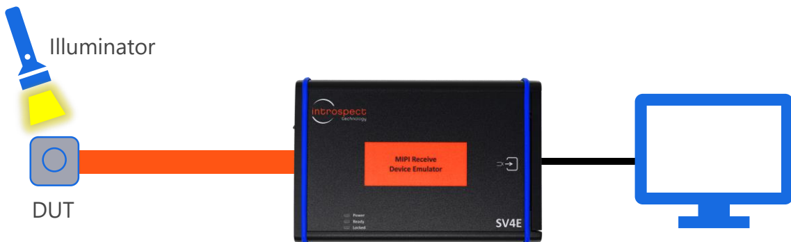
Figure 2. SV4E-DPRXCPRX testing a C-PHY camera module
